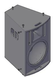
For suspended installation, there are six brackets inside the case: three in the top, three in the bottom. Each bracket is secured to two adjacent internal side of speaker using two M10 screwbolts.
